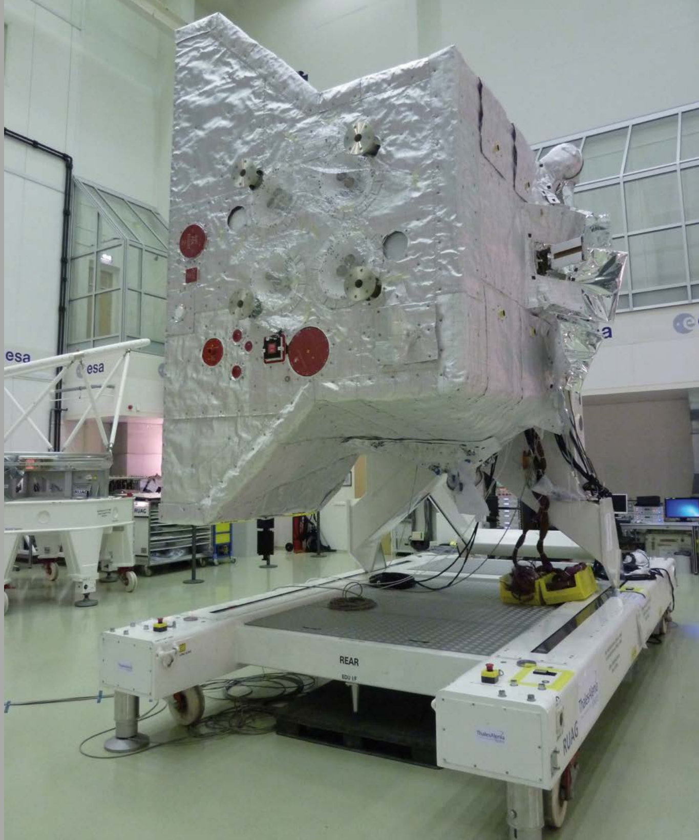
BepiColombo Mercury Planetary Orbiter Flight Model spacecraft in final preparation for thermal test at ESTEC
