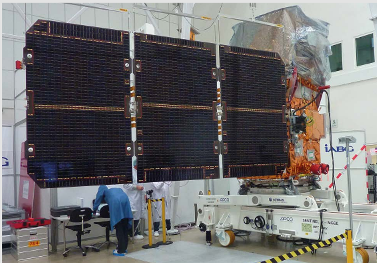
Sentinel-2A solar array deployment test at IABG (Airbus Defence & Space)
